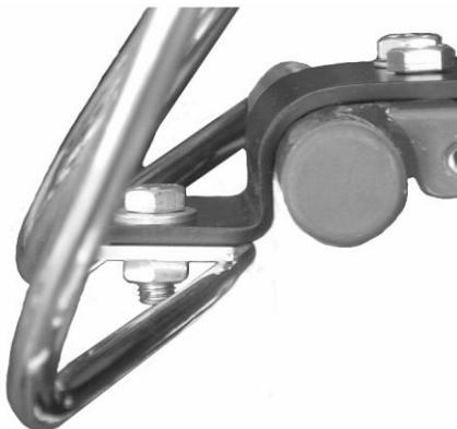
**3.** Raise the accessory to align the rear brackets to the Mounting Plate holes and insert the thin-head bolts and washers.
