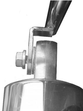
3. Raise the accessory to align the rear mounts to the Mounting Plate holes and insert the thin-head bolts and washers.
